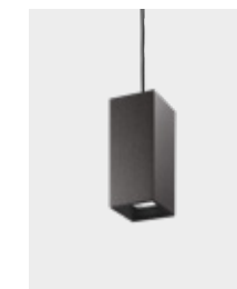
Altopiano S 1.1 power: 8W optics: 50° colour temp.: 3000K finish: cor-ten
