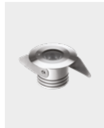
Beam 1.0 power: 3W optics: 8° colour temp.: 2700K finish: stainless steel
