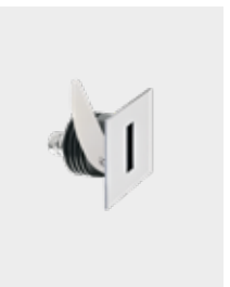
Step Outside 6.3 power: 2W optics: asymmetrical colour temp.: 3000K finish: satin
